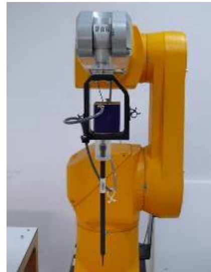
Figure 3. EX3DV4 E-field probe
