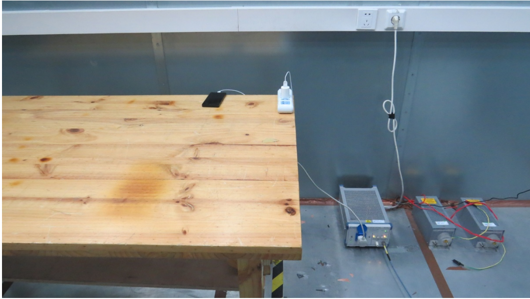
Picture 3 Conducted Emission Test Setup
