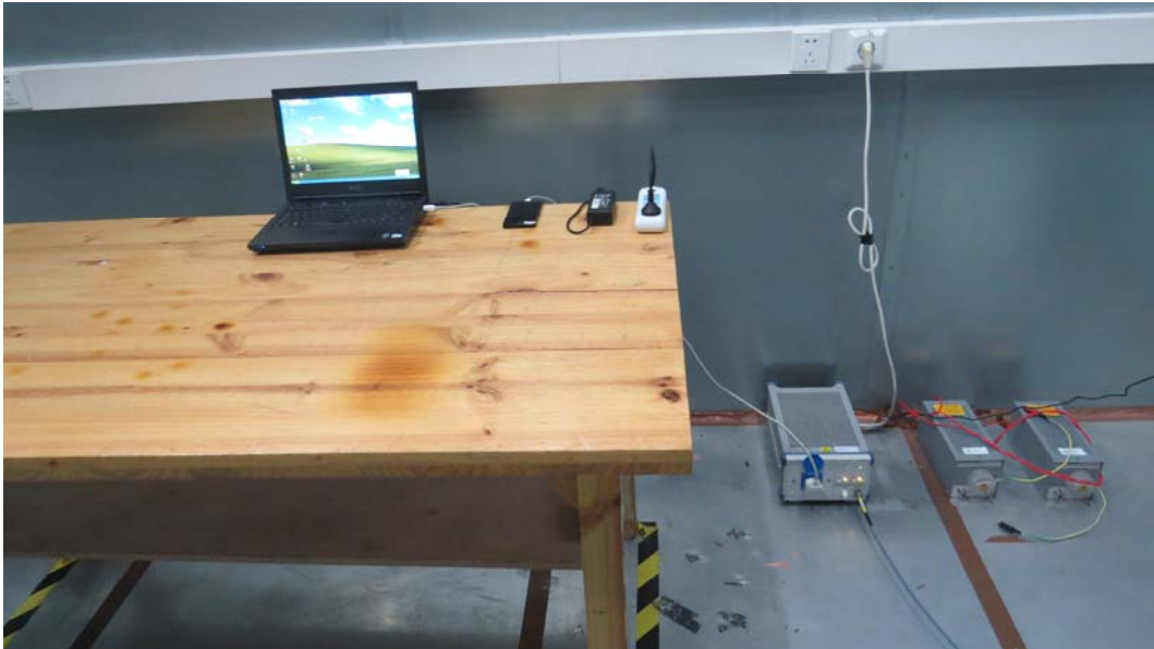
Picture 3 Conducted Emission Test Setup
