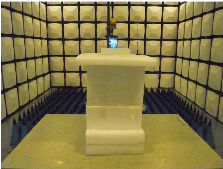
Radiated Emission View---Above 1GHz
