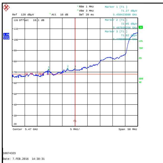
Lower Band Edge Measurement
