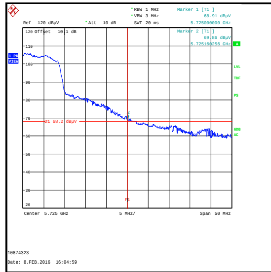
Upper Band Edge Measurement
