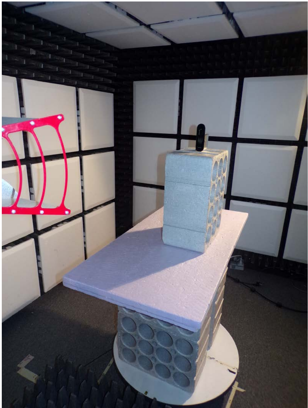
Test setup for radiated emission above 1GHz
