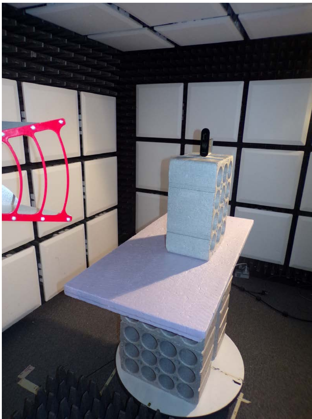
Test setup for radiated emission above 1GHz
