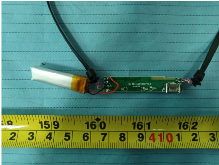
EUT –Main Board & Battery Bottom View
