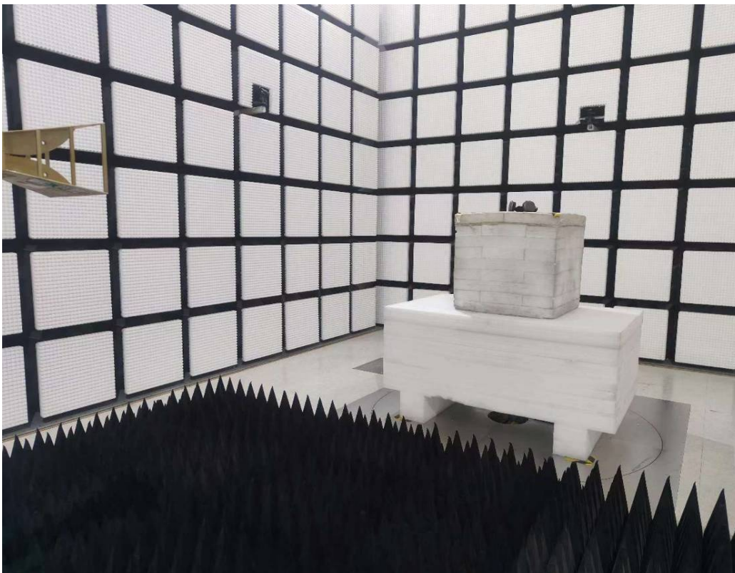
Radiated Emission Above 1GHz View
