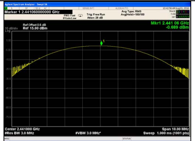
GFSK Output power - Mid CH 2441
