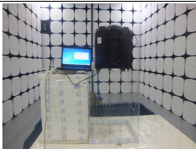
Radiated Spurious Emissions Test Above 1GHz
