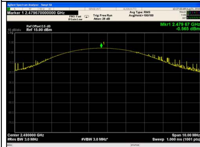
8DPSK Output power - High CH 2480
