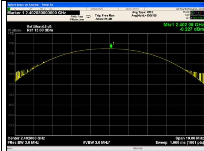
GFSK Output power - Low CH 2402
