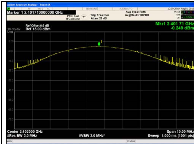
8DPSK Output power - Low CH 2402
