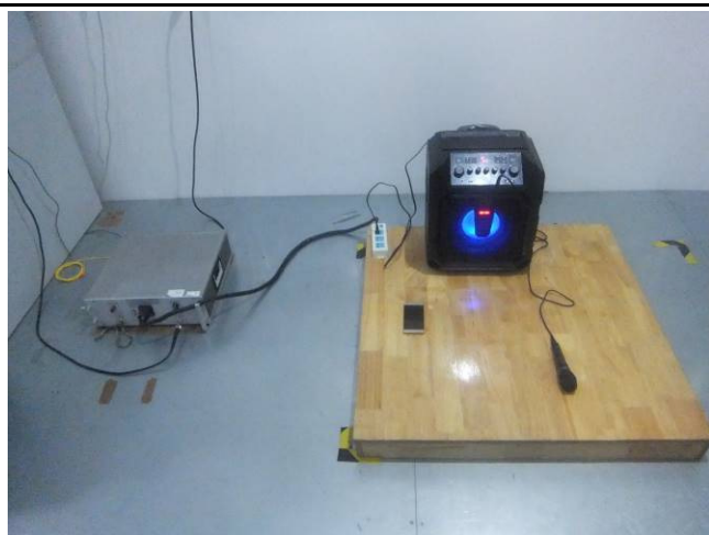
Conducted Emissions Test Setup – Front View
