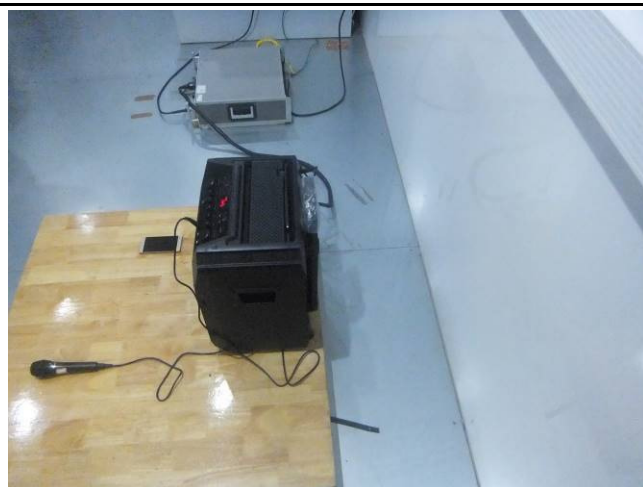
Conducted Emissions Test Setup – Side View
