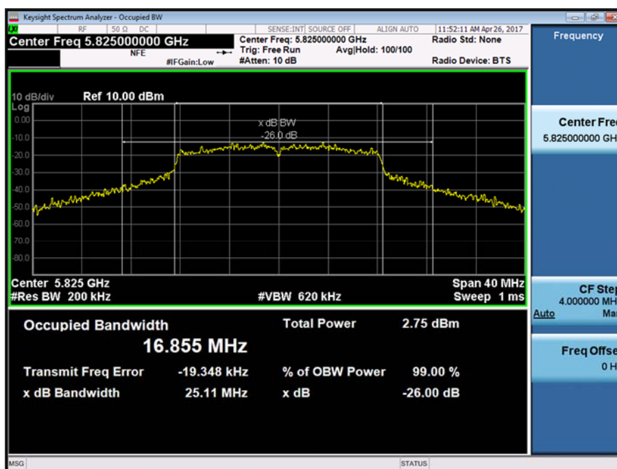
Figure 14 - U-NII 3 - 5825 MHz - 6 dB Bandwidth
