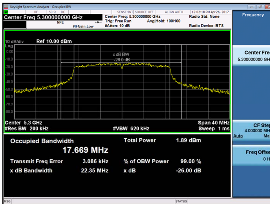
Figure 19 - U-NII 2a - 5300 MHz - 26 dB Bandwidth
