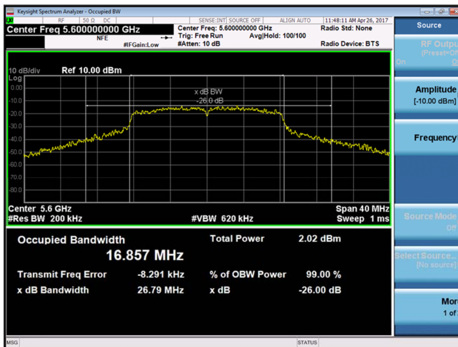
Figure 10 - U-NII 2c - 5600 MHz - 26 dB Bandwidth
