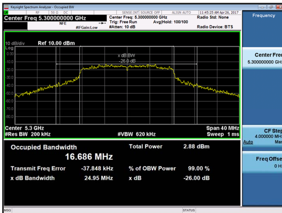
Figure 7 - U-NII 2a - 5300 MHz - 26 dB Bandwidth
