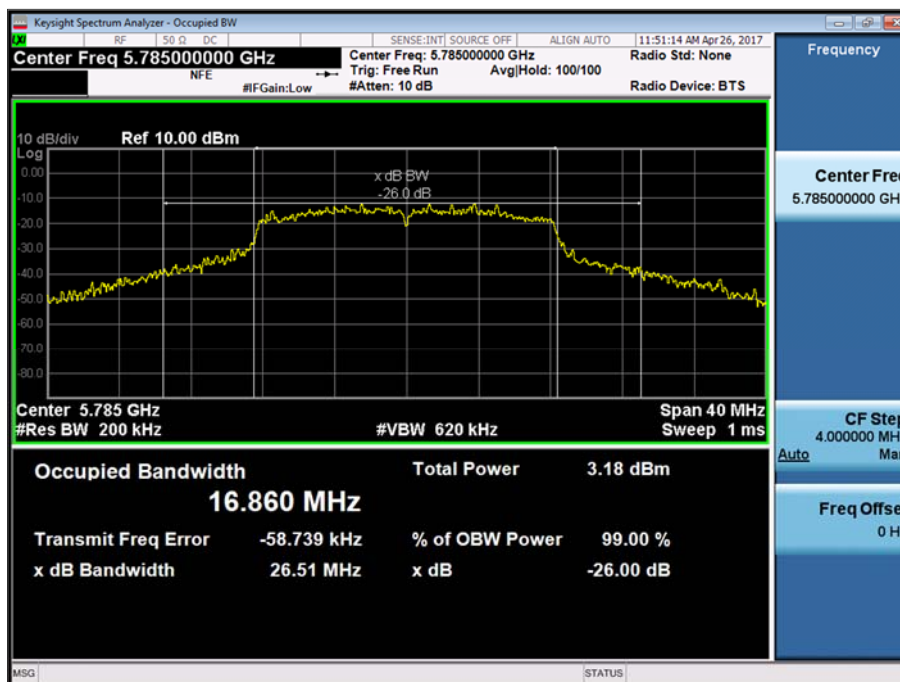
Figure 13 - U-NII 3 - 5785 MHz - 6 dB Bandwidth
