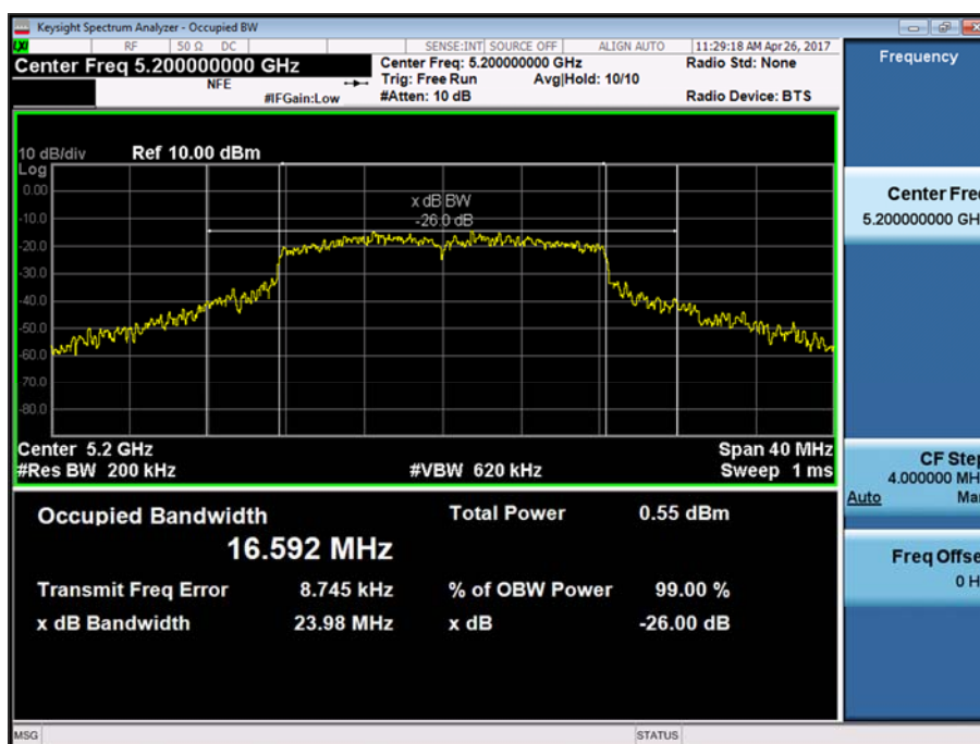
Figure 4 - U-NII 1 - 5200 MHz - 26 dB Bandwidth
