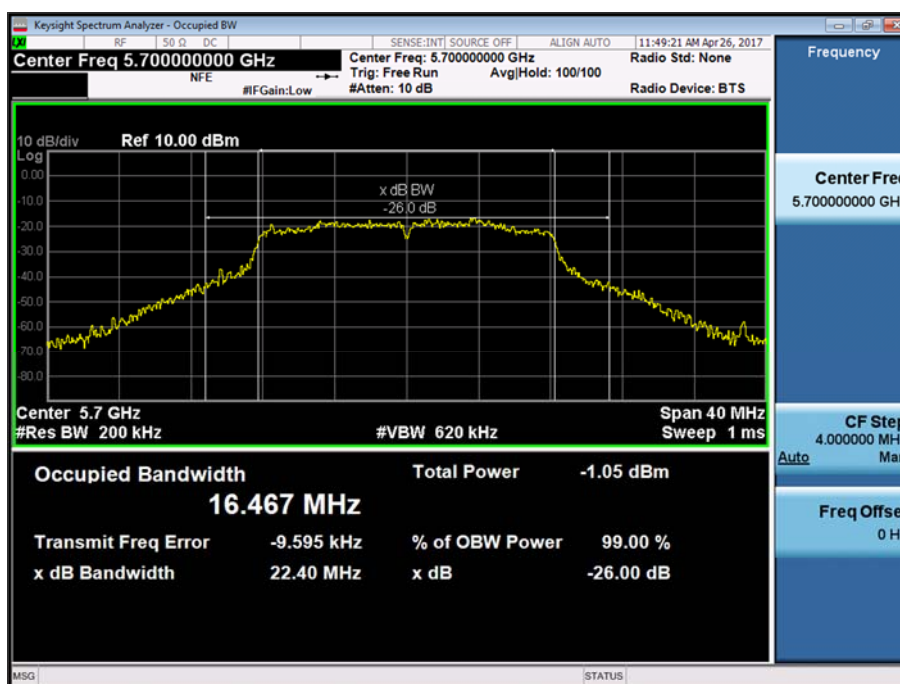
Figure 11 - U-NII 2c - 5700 MHz - 26 dB Bandwidth
