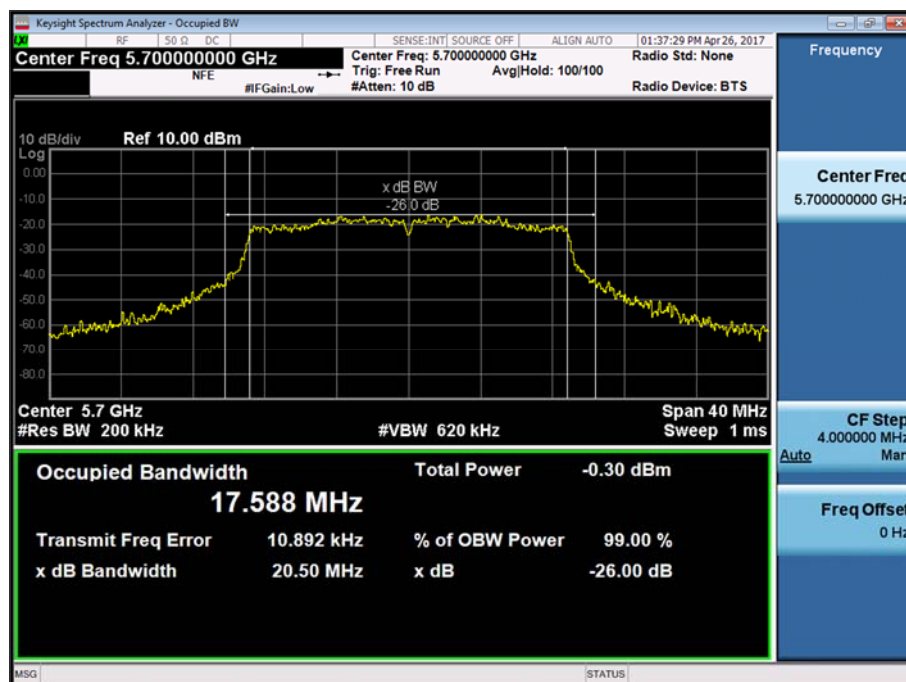
Figure 44 - U-NII 2c - 5700 MHz - 26 dB Bandwidth
