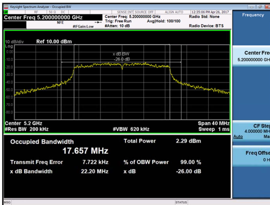
Figure 37 - U-NII 1 - 5200 MHz - 26 dB Bandwidth
