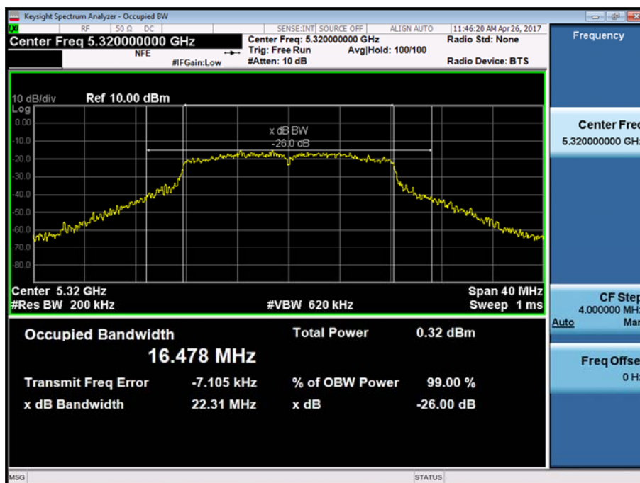
Figure 8 - U-NII 2a - 5320 MHz - 26 dB Bandwidth
