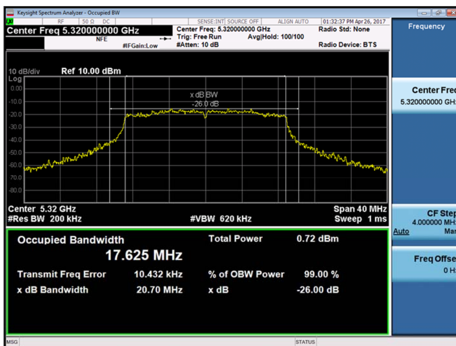
Figure 41 - U-NII 2a - 5320 MHz - 26 dB Bandwidth
