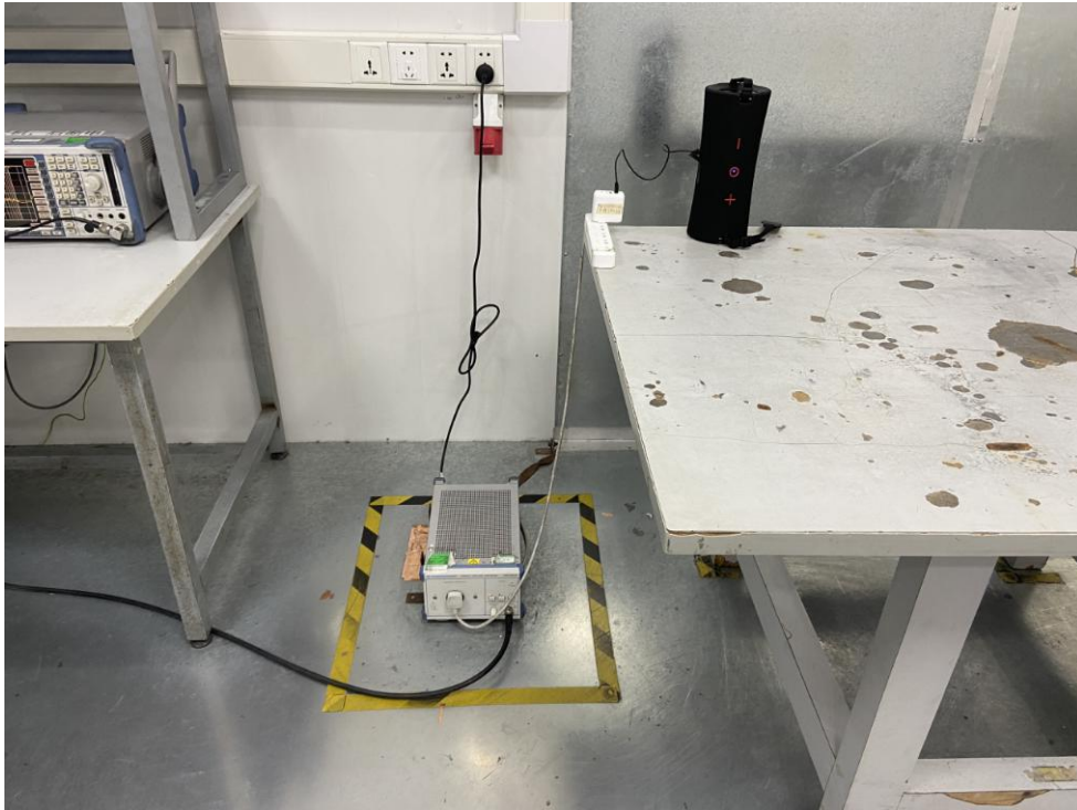
FCC ID: 2AEX7-AD-SPK1 Photo of Power Line Conducted Emission Test
