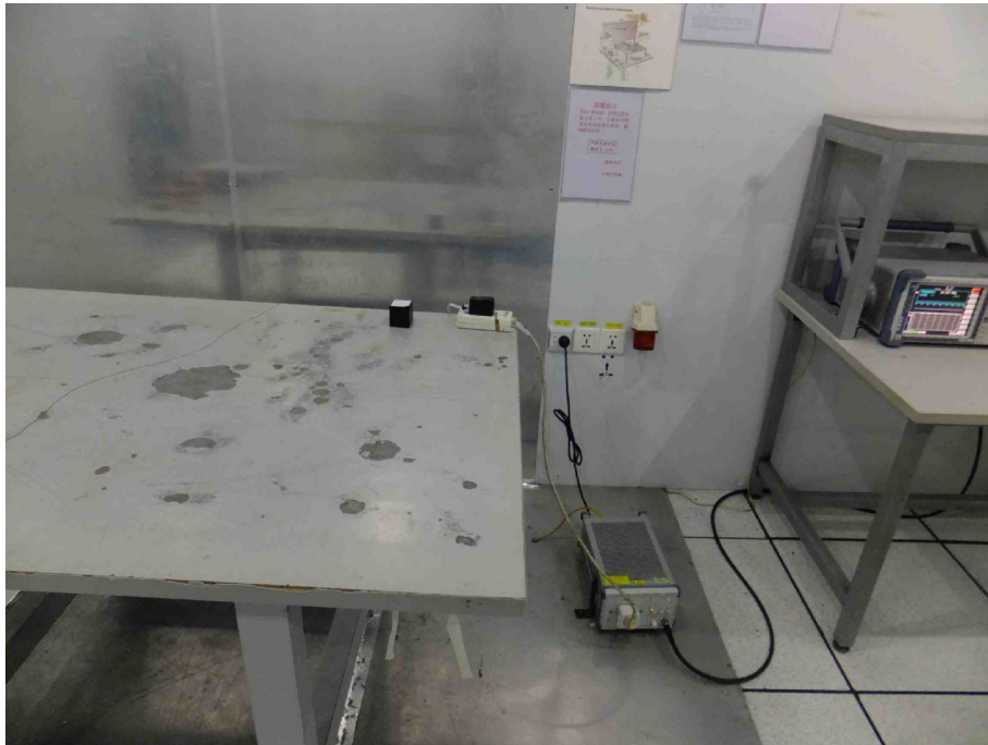
1 Photo of Power Line Conducted Emission Measurement
