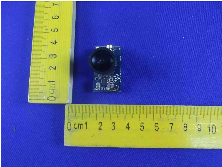
Figure 13 PCB of the EUT-Front View
