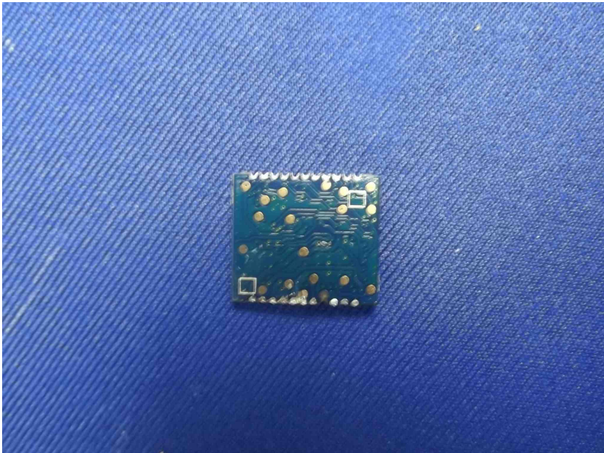
Figure 21 PCB of the EUT-Back View
