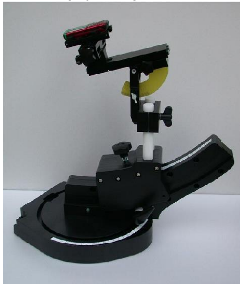
Device holder supplied by SPEAG
