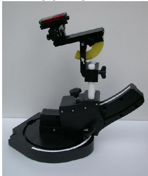
Device holder supplied by SPEAG
