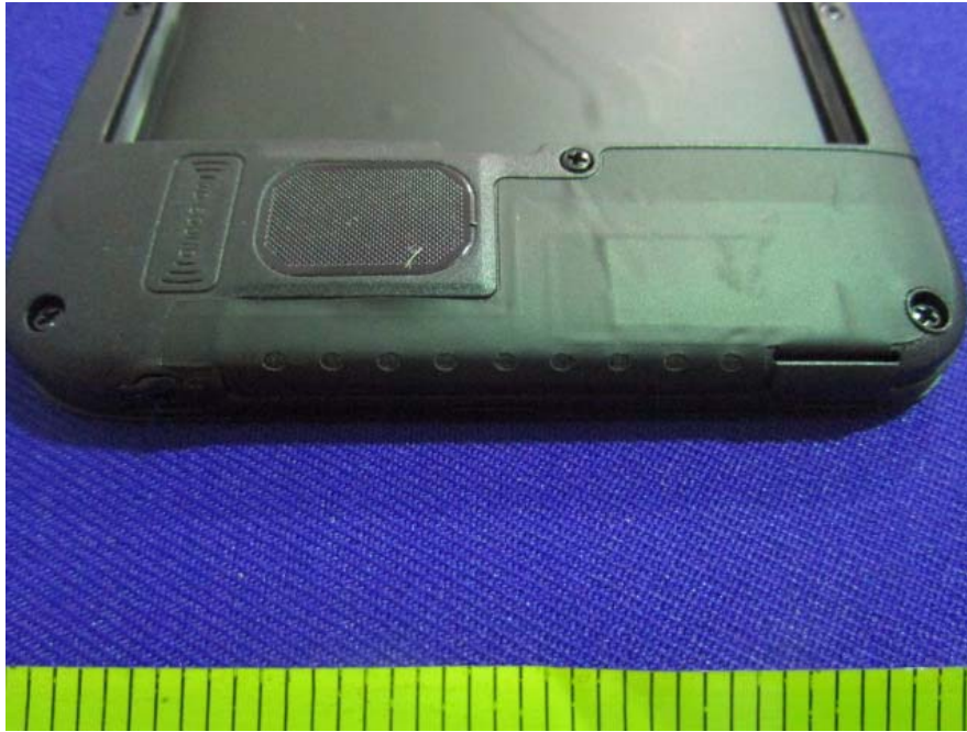
EUT –GSM&WCDMA&LTE Main Antenna View
