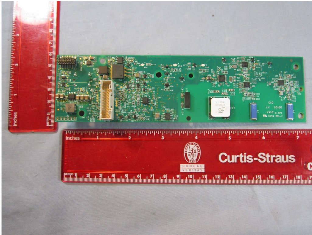
Front of Internal Board
