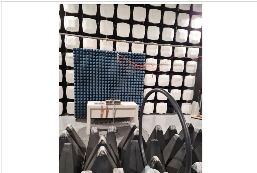
Photograph 2: EUT test setup in the fully anechoic chamber, Radiated field strength emissions below 30 MHz
