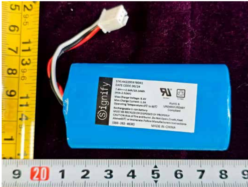
FIGURE 17 COMBO EXIT SIGN WITH FIRSTLINK (BCB4WFL1) BATTERY
