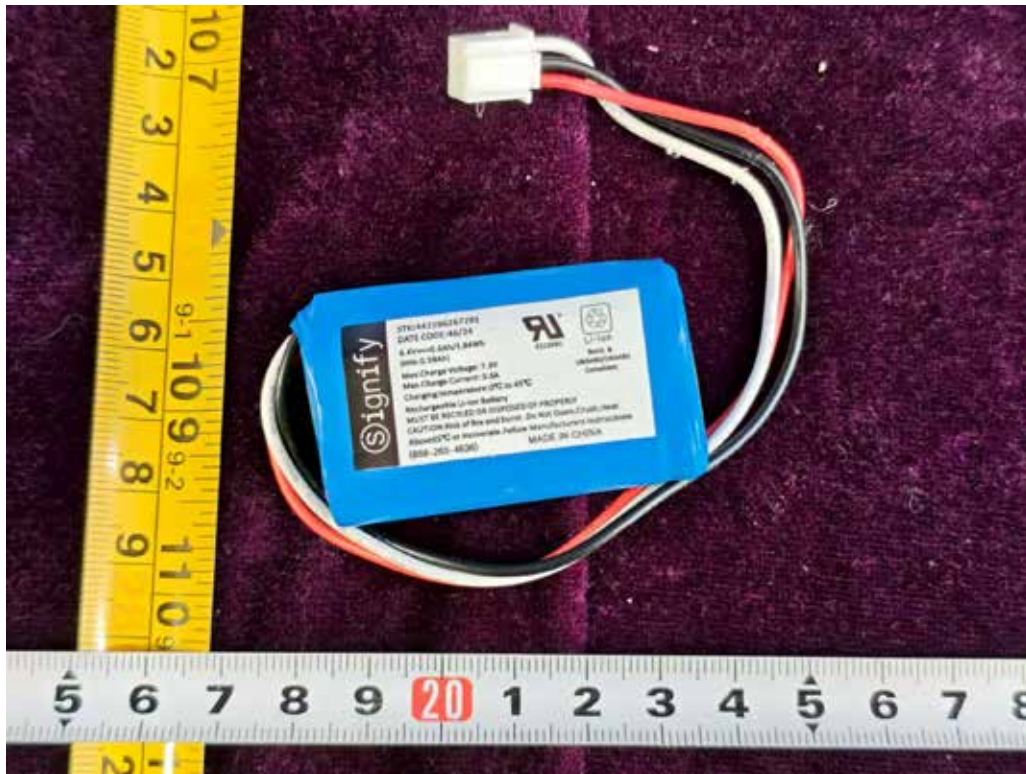
FIGURE 30 EXIT SIGN WITH FIRSTLINK (BxBWFL1) BATTERY
