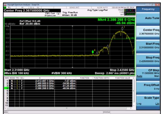
,Plot 2,Band Edge-802.11b,2462MHz
