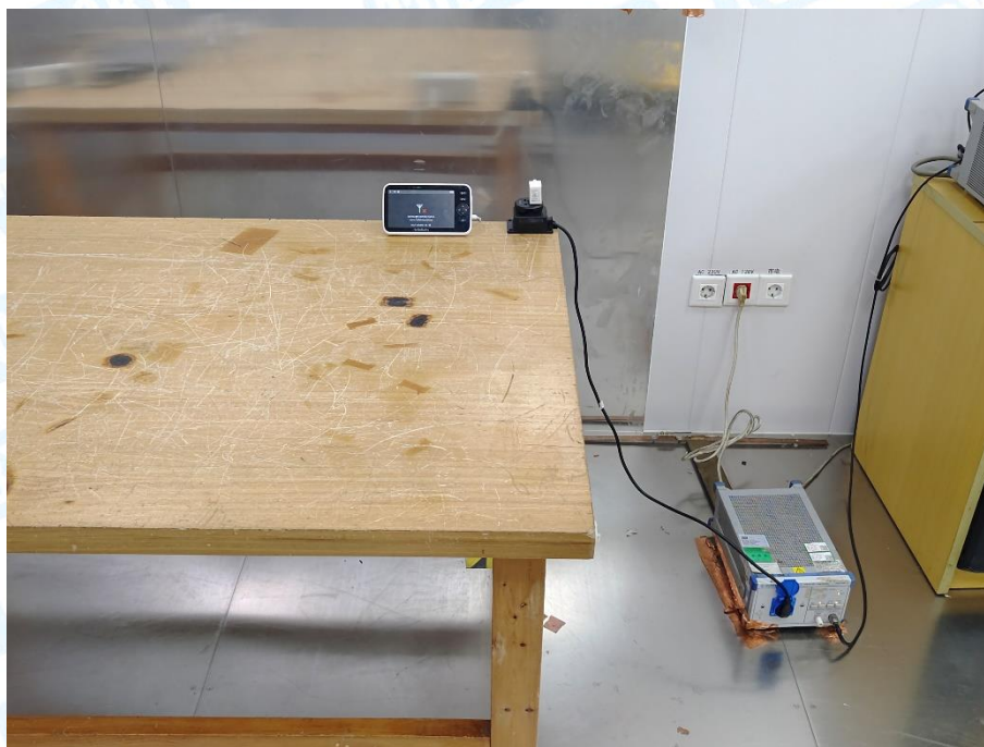
Photo of Setup for Conducted Emission
