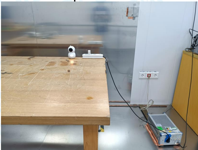
Photo of Setup for Conducted Emission
