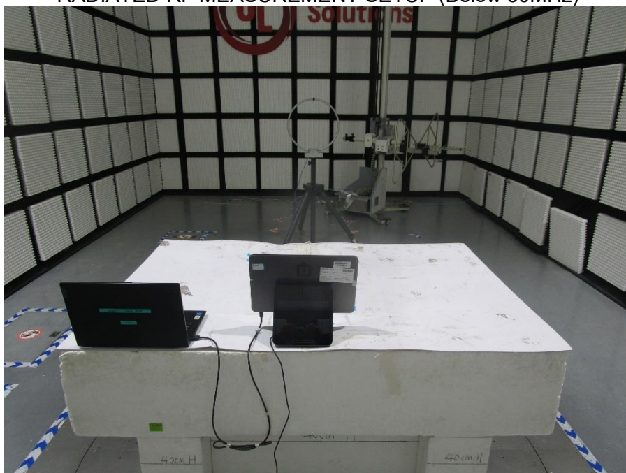
RADIATED RF MEASUREMENT SETUP (Below 30MHz)
