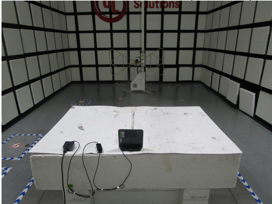
RADIATED RF MEASUREMENT SETUP (30MHz~1GHz)
