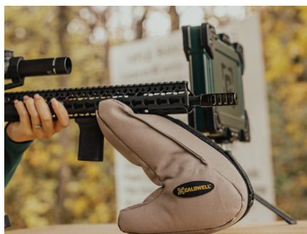
VELOCIRADAR SLIGHTLY BEHIND MUZZLE.
