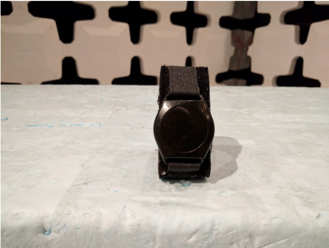
Figure 8 – EUT position, Y-axis
