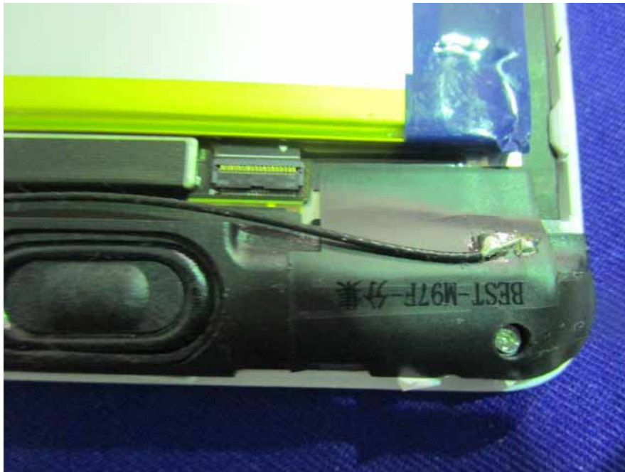
EUT –LTE Diversity Antenna View
