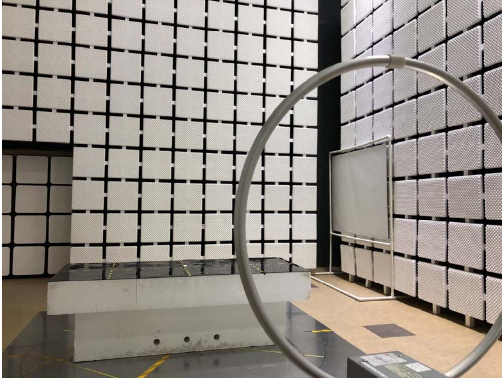
Radiated RF measurement (Below 30 MHz)
