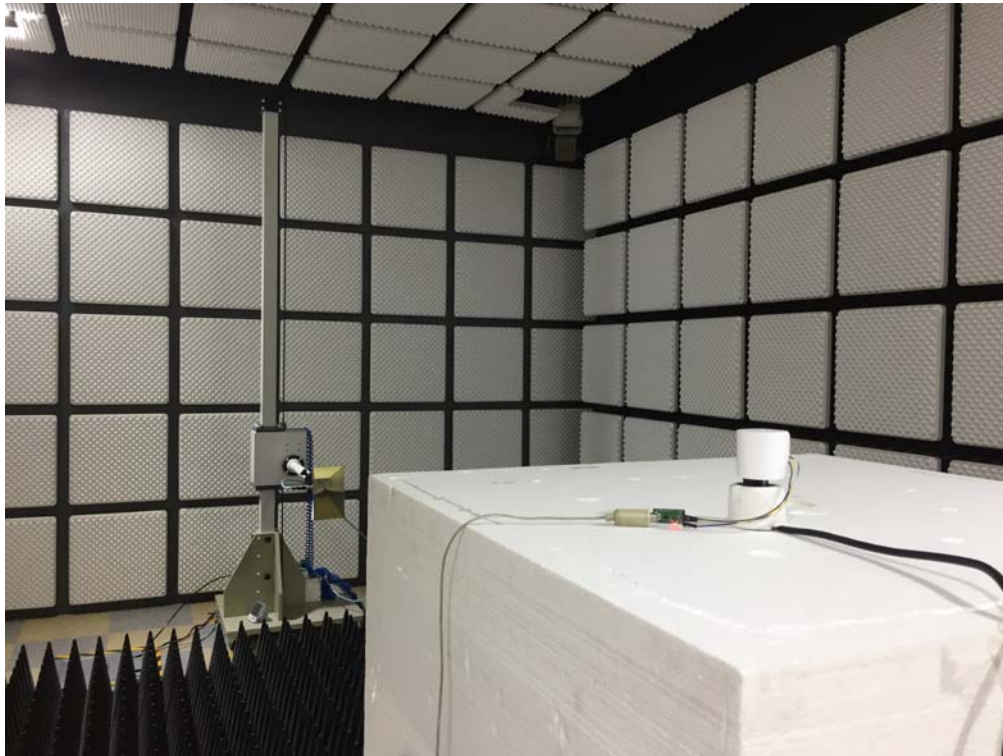
Radiated RF measurement (Above 1 GHz)
