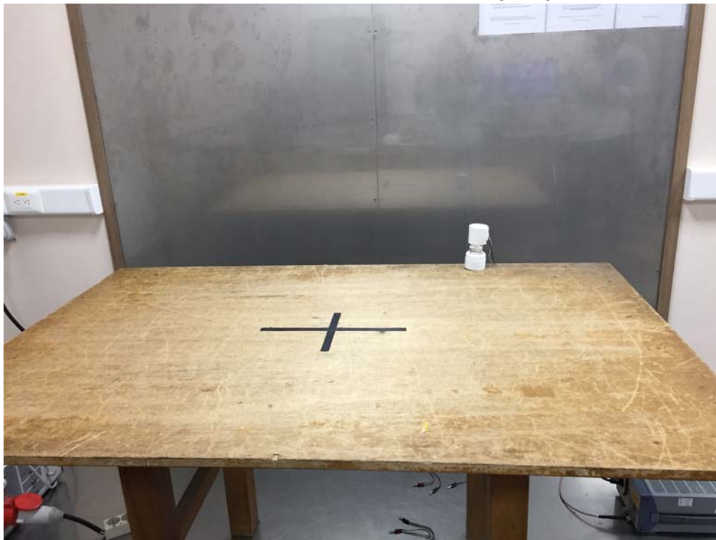
Conducted Emission measurement (front)
