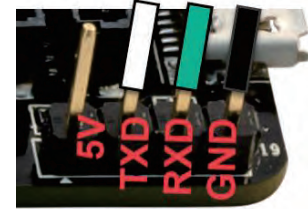
J19 USB-Serial cable to SCIF0 connections
