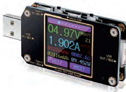
Figure 7 – Current-measurement USB Dongle
