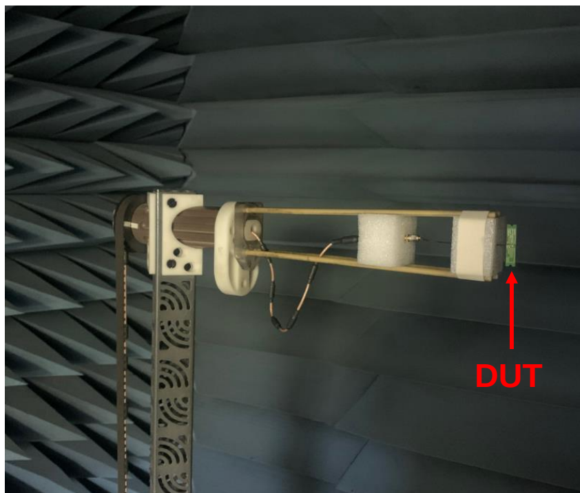
FIGURE4.1.2 ANTENNA IN FREE SPACE WITH OTA CHAMBER
