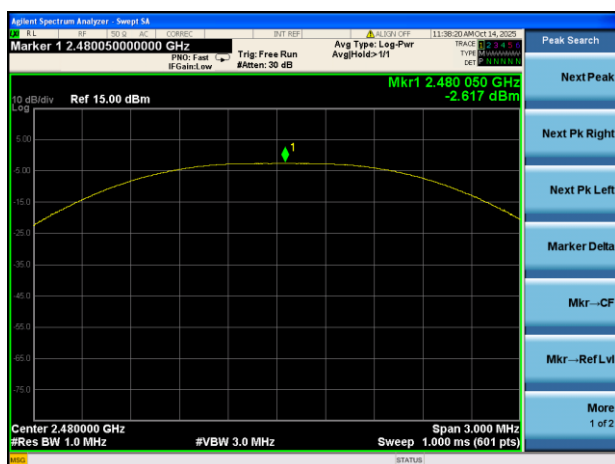
GFSK (BLE 1Mbps) HIGH CHANNEL
