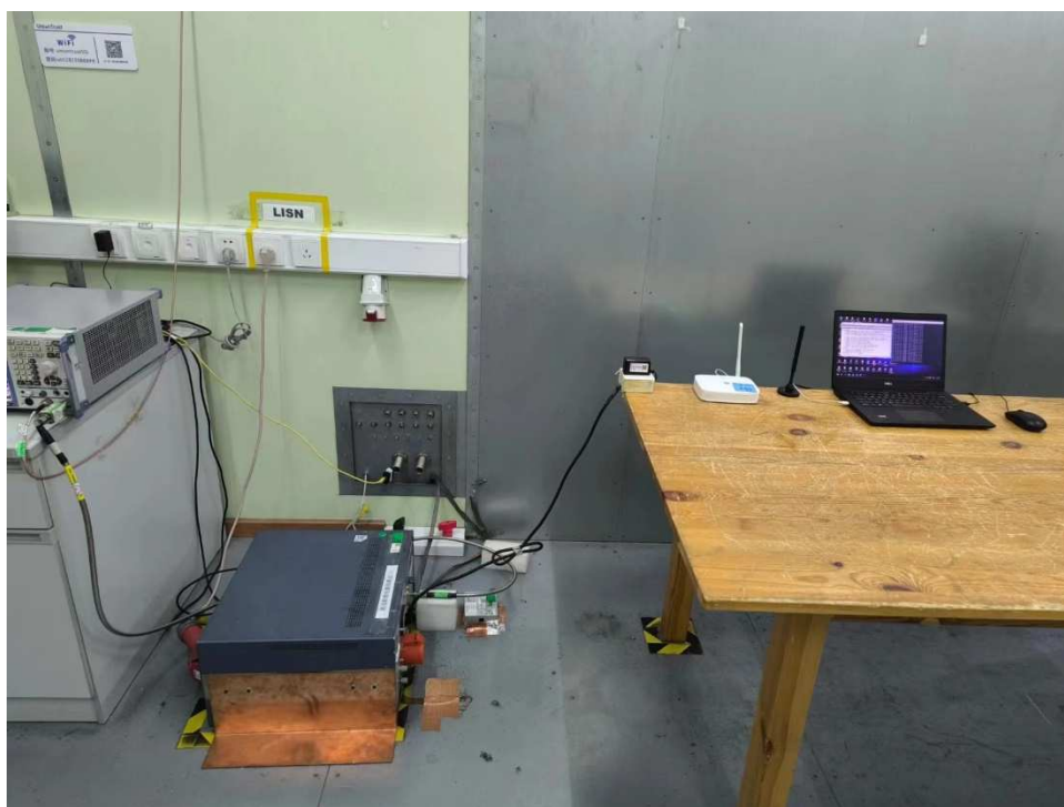
Photograph 3: Set-up for Conducted Emissions, AC Mains
