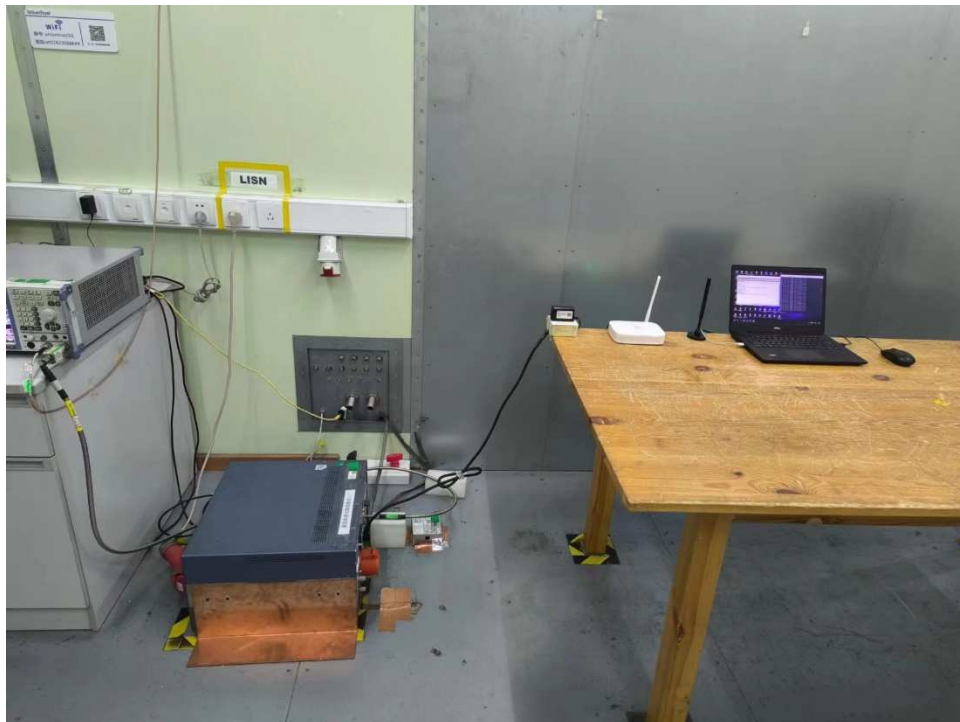
Photograph 3: Set-up for Conducted Emissions, AC Mains
