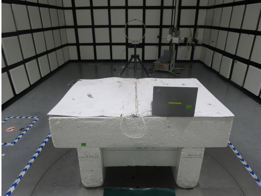
RADIATED RF MEASUREMENT SETUP (Below 30MHz)
