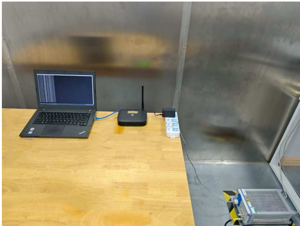
Photograph 3: Set-up for Conducted Emissions, AC Mains
