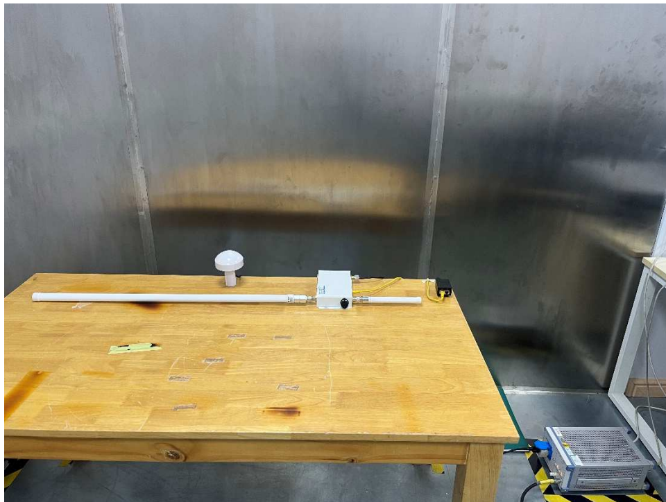
Photograph 1: Set-up for Conducted Emissions, AC Mains
