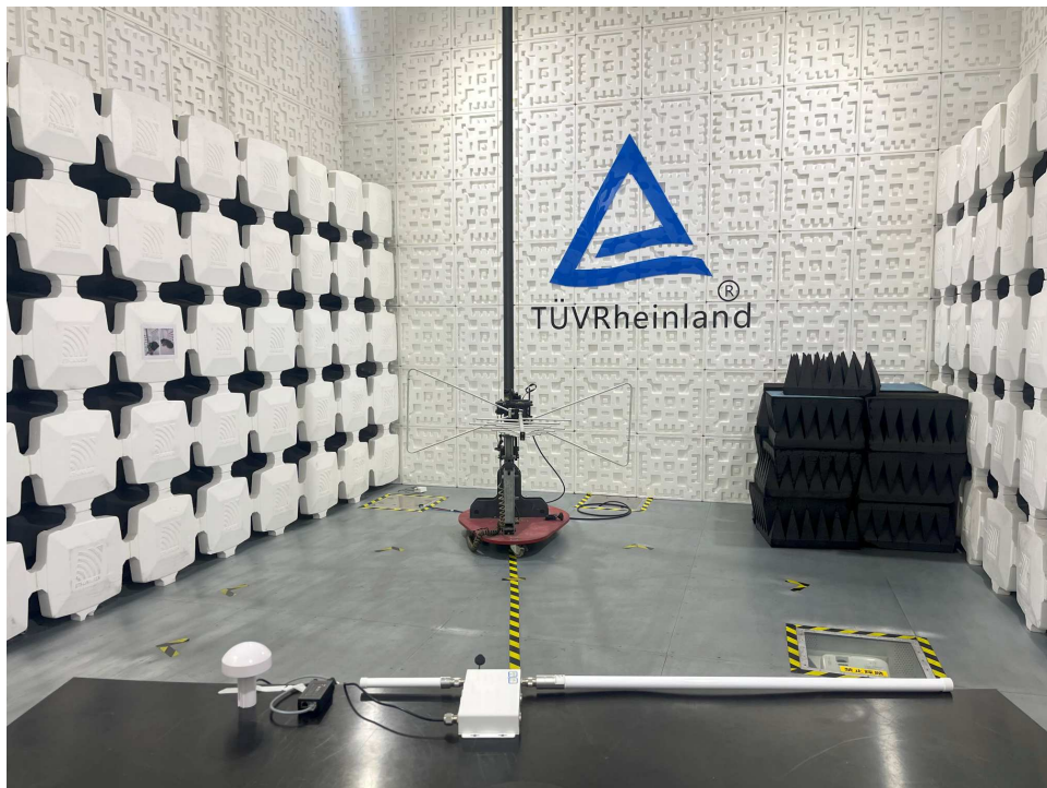
Photograph 2: Set-up for Radiated Emissions, below 1GHz
