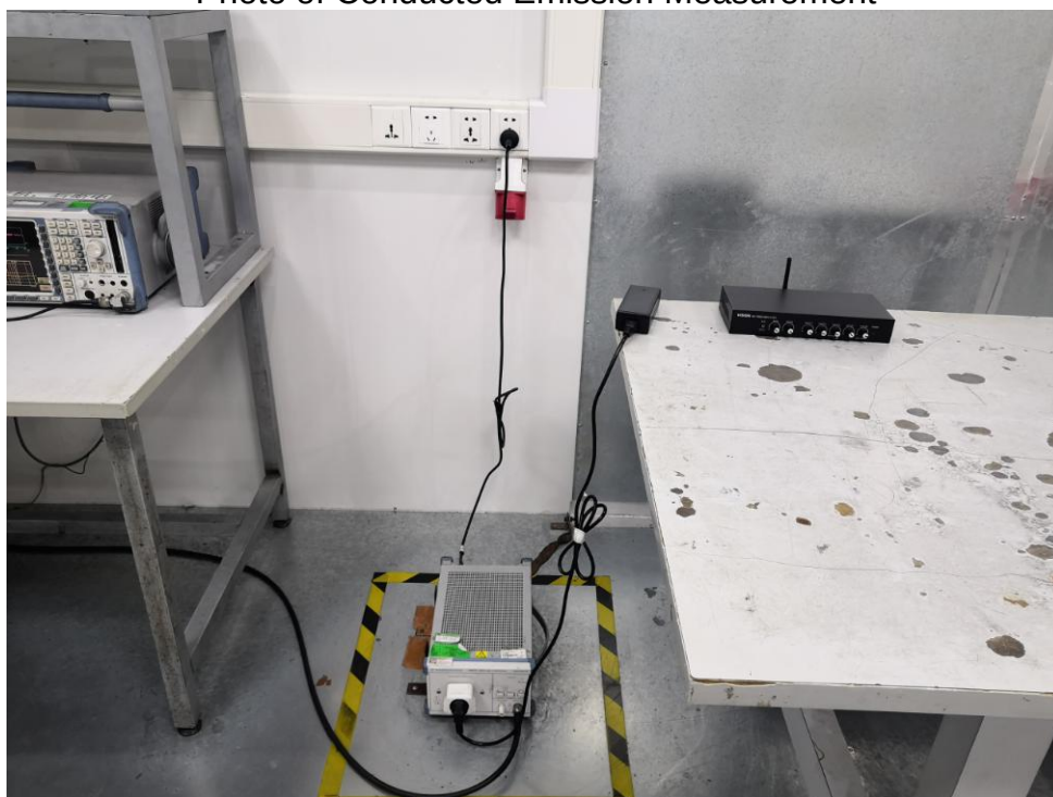
FCC ID: 2AF6C-AV-1900 Photo of Conducted Emission Measurement
