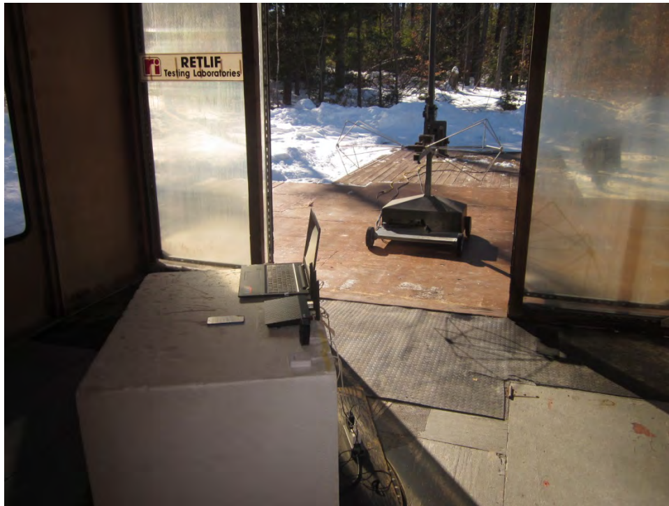
Horizontal Antenna Polarization, 30 MHz – 200 MHz
