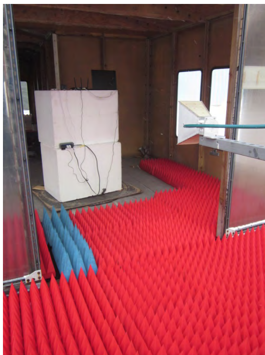
Horizontal Polarization, 1- 12 GHz, Double Ridge Guide, 150 cm
