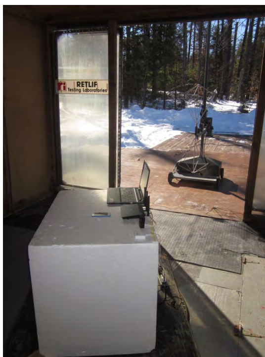
Vertical Polarization, 30 MHz – 200 MHz, Biconical Antenna, 80 cm
