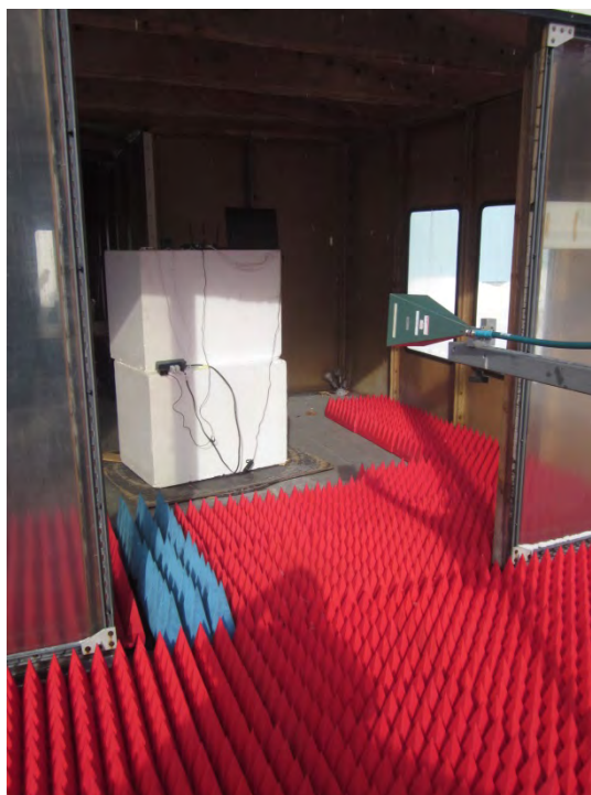
Horizontal Polarization, 12- 18 GHz, High Gain Horn, 150 cm
