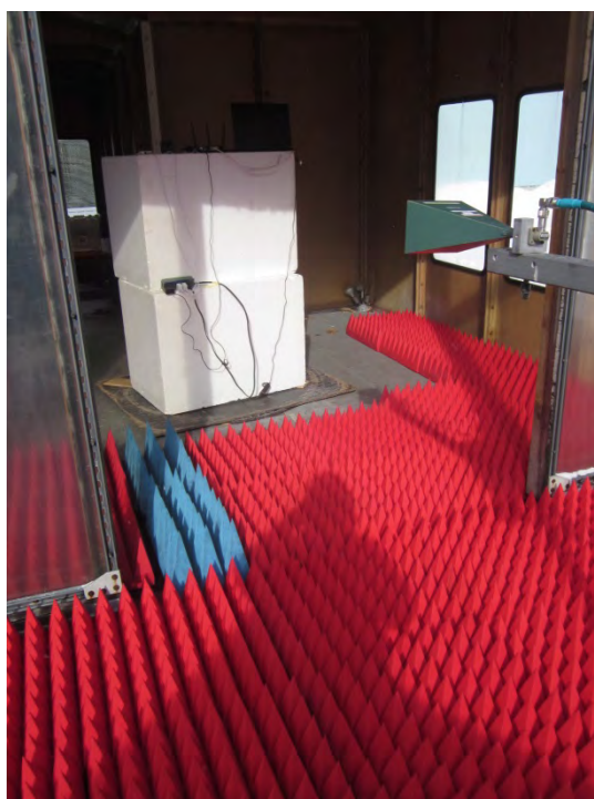
Vertical Polarization, 12- 18 GHz, High Gain Horn, 150 cm
