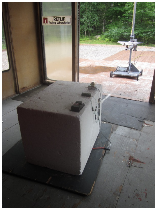
Horizontal Antenna Polarization, 200 MHz to 1 GHz
