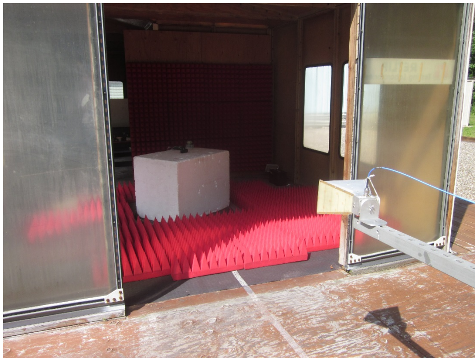
Vertical Antenna Polarization, 1 GHz to 10 GHz
