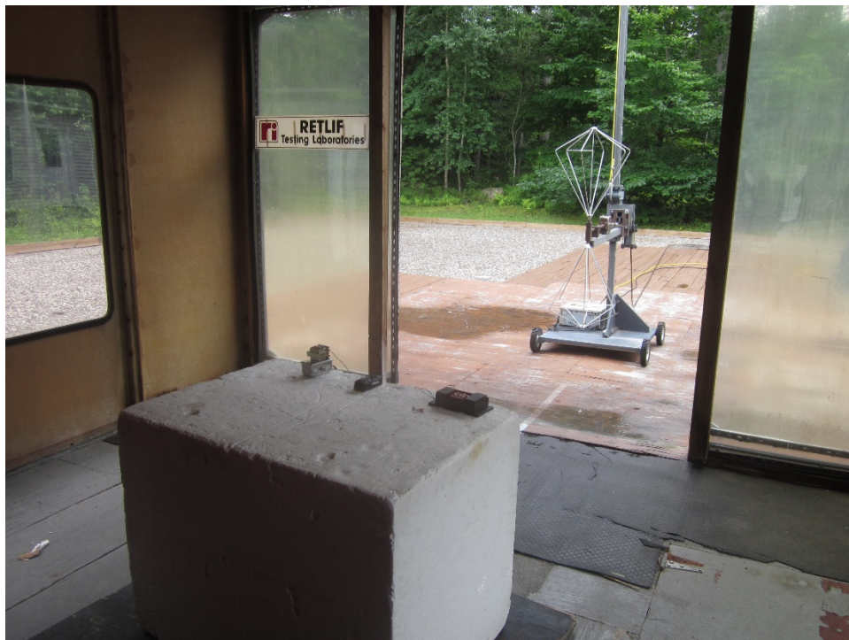
Vertical Antenna Polarization, 30 to 200 MHz
