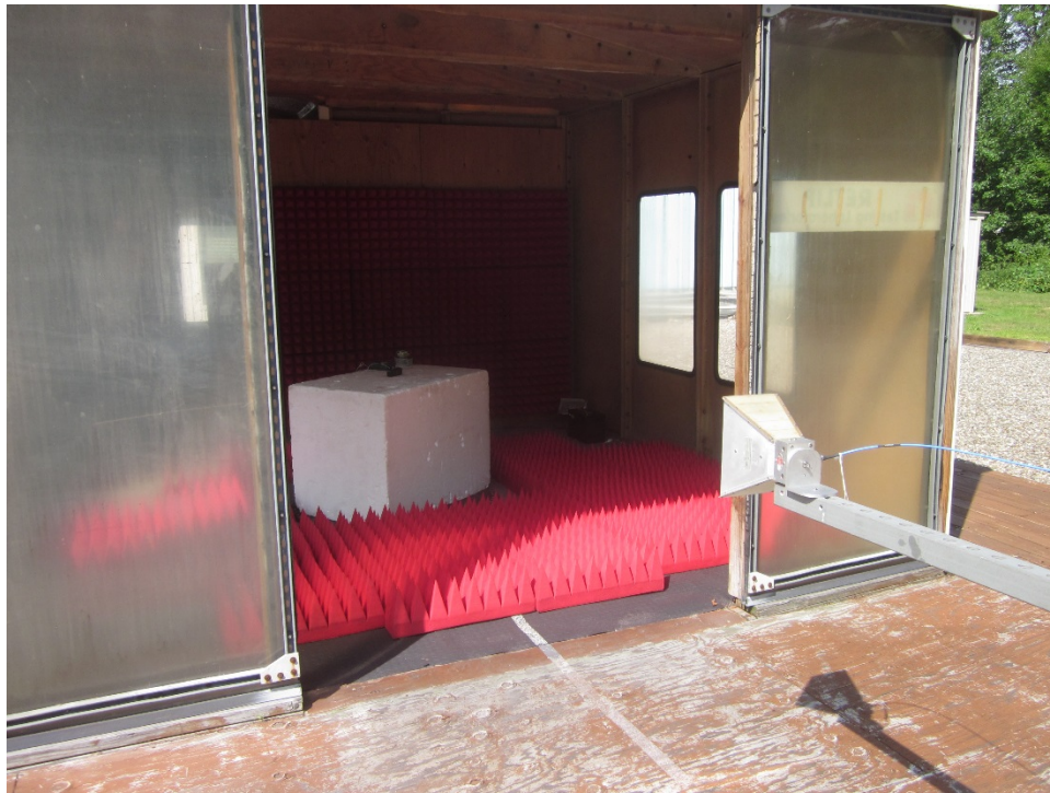
Horizontal Antenna Polarization, 1 GHz to 10 GHz
