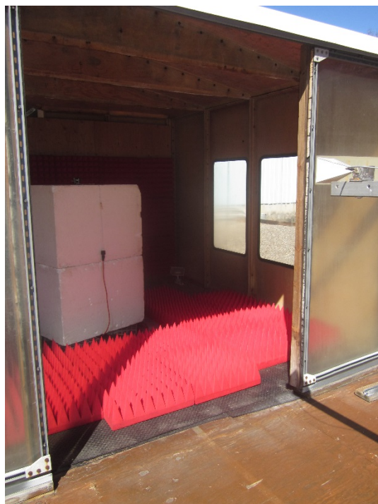
Horizontal Polarization, 18 to 25 GHz, High Gain Horn, 150 cm
