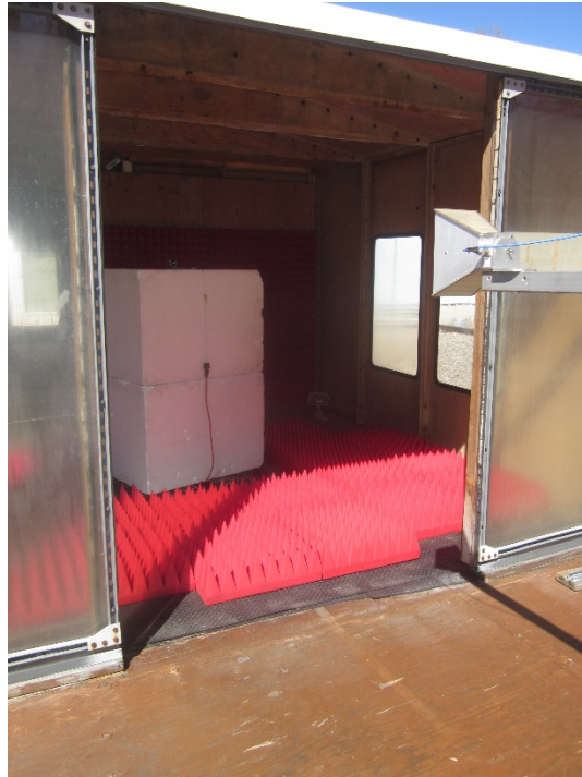
Horizontal Polarization, 1 to 18 GHz, Double Ridge Guide, 150 cm
