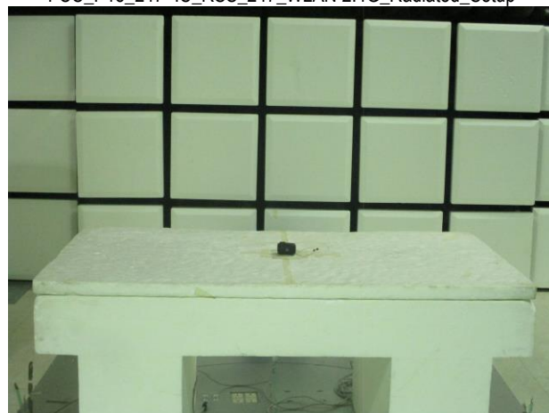
FCC_P15_247+IC_RSS_247_WLAN 2.4G Radiated_Setup
