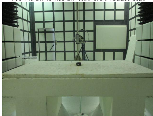
FCC_P15_247+IC_RSS_247_WLAN 2.4G Radiated_Setup
