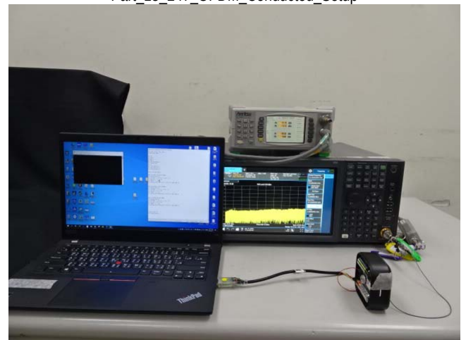
Part 15 247 OFDM Conducted Setup
