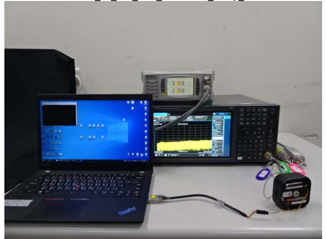
Part 15 247 FSK Conducted Setup_2
