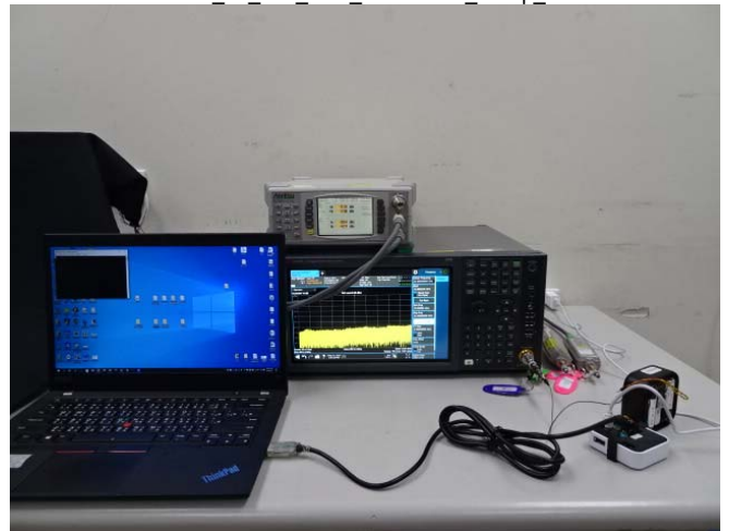
Part 15 247 FSK Conducted Setup_2
