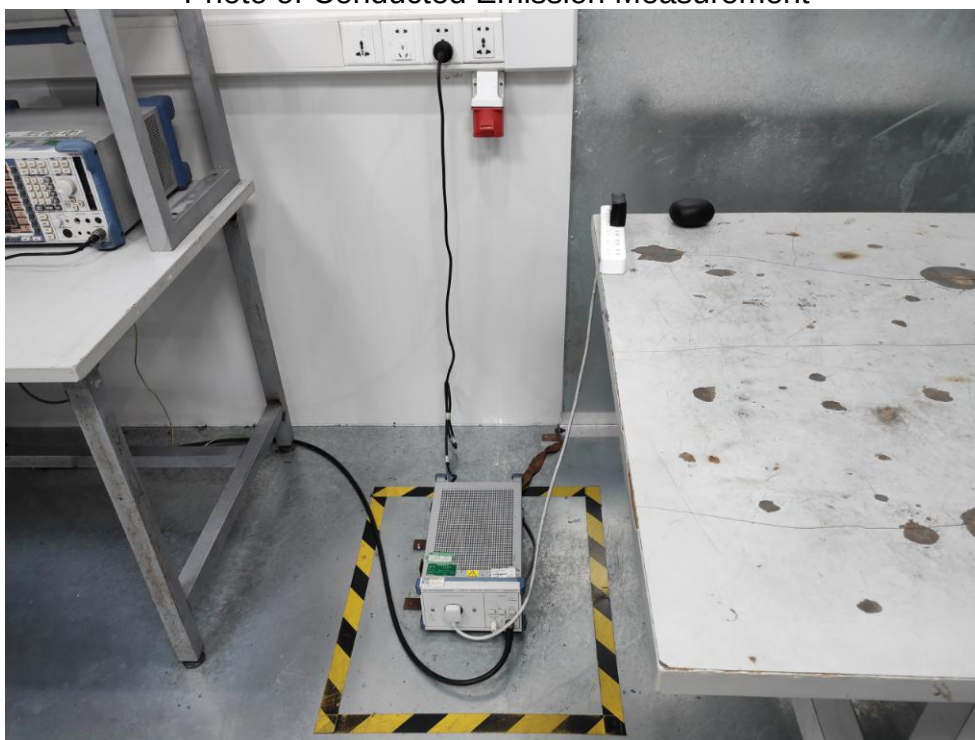
FCC ID: 2AF8Q-JT05 Photo of Conducted Emission Measurement
