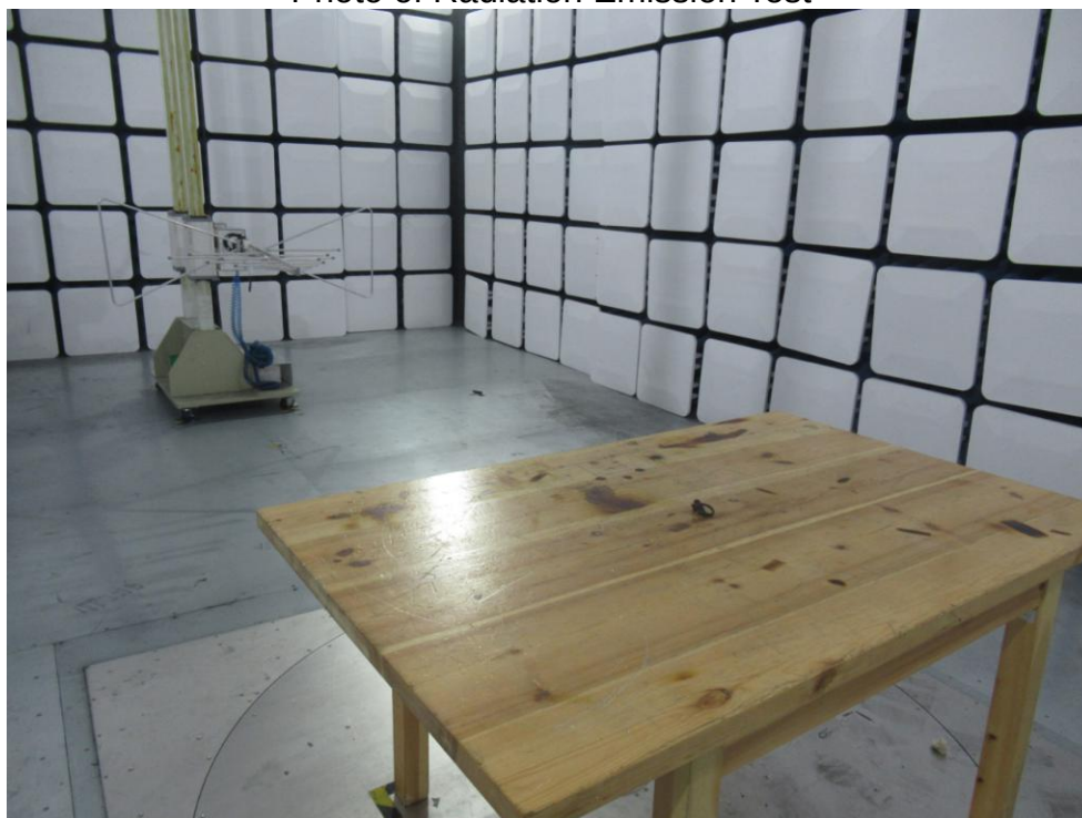
Photo of Radiation Emission Test
