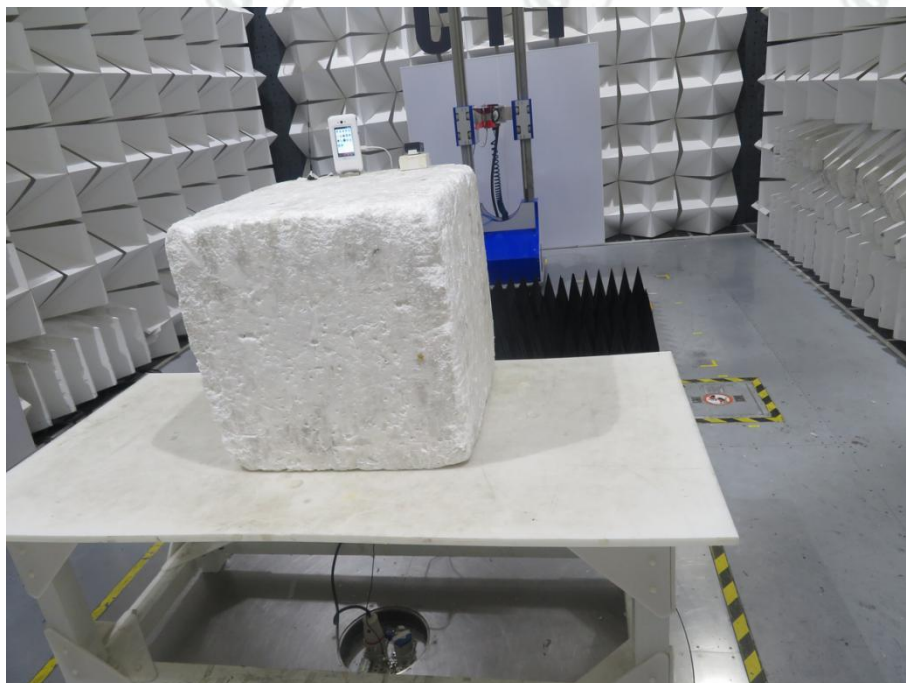
Radiated spurious emission Test Setup-2(Above 1GHz)
