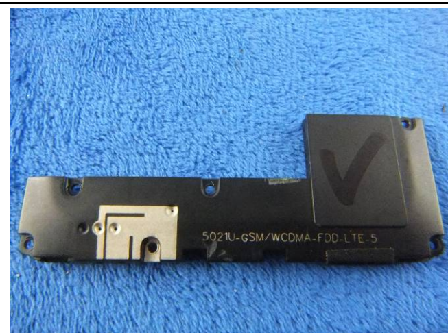
GSM/PCS/UMTS-FDD Antenna View
